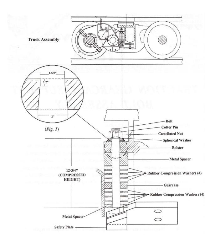
Never lay under the Gear Case or Motor while servicing this support!
