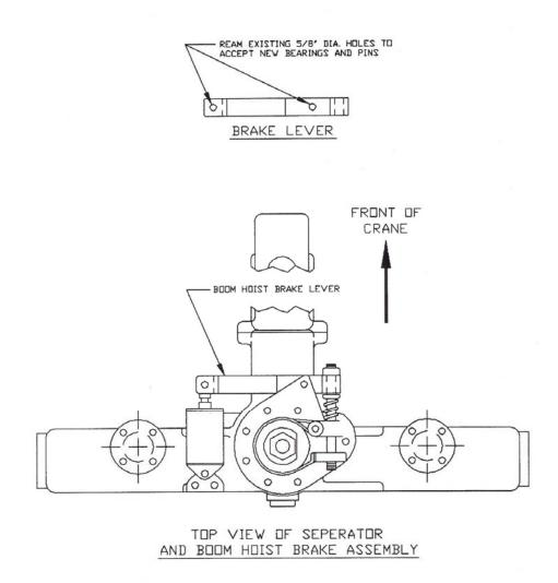
Boom Hoist Brake Band Assembly should be periodically inspected for wear and cracking.
